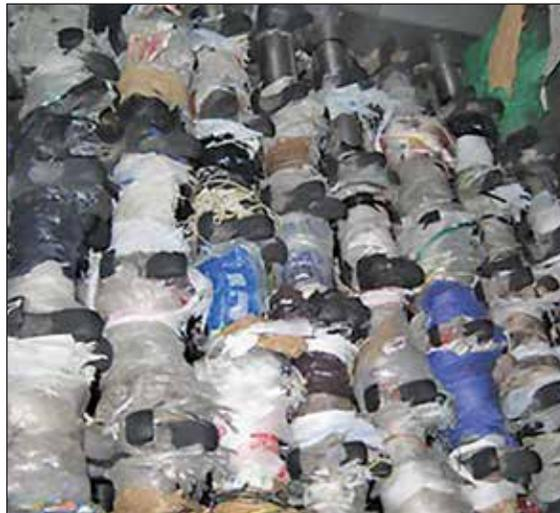
Photo (left) is a typical problem for many recycling facilities. Shown here are plastic bags and soft plastics tangled in the sorting conveyors. When this happens, it can damage machinery if the plastics are not cleared out before continuing.
