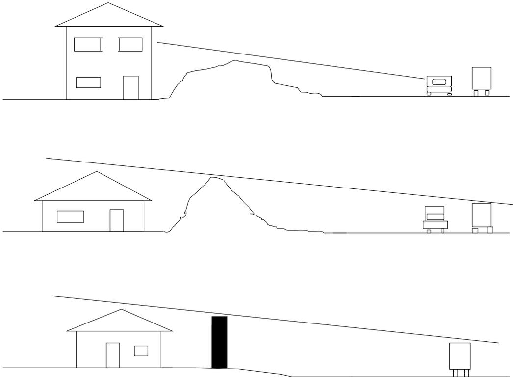
Noise impacts can be reduced by the use of a single story house. To be effective, a barrier must block the line of sight between the highest point of a noise source and the highest point of a receiver.
